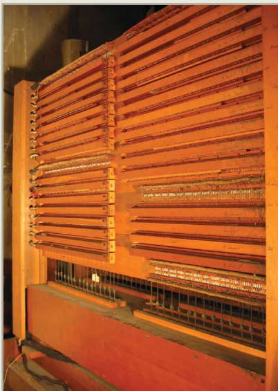
Some of Orpheum’s stop relays, which are housed in the Main chamber.
