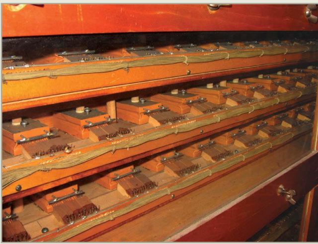
Some of Orpheum's key relays are visible behind glass front of the pressurized case that holds them.
